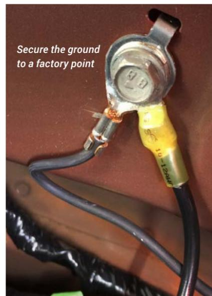
Secure the ground to a factory point
