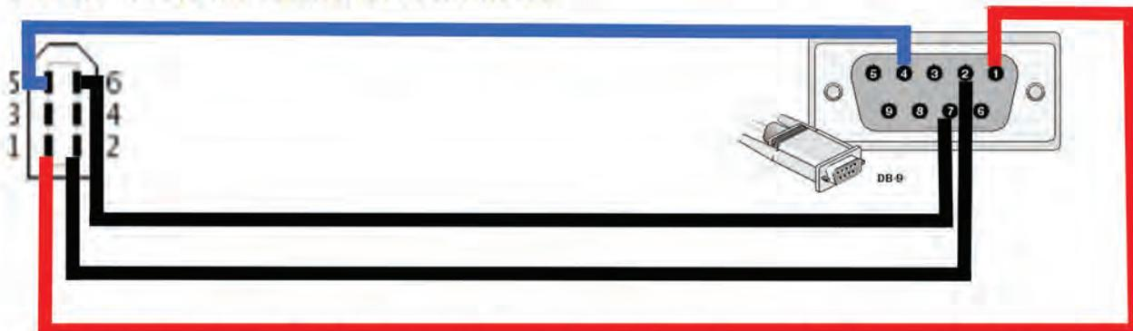
JMS has two different EGT Cable Options. 9617A - utilizes a DB9 cable to Firewire (shown). 9617B - utilizes an integrated cable on the EGT box side to Firewire. Both wire the same. Firewire Pin 1 = +5V, Pin 2 = Ground, Pin 5 = EGT Signal (0-5V), Pin 6 = EGT Signal Ground
