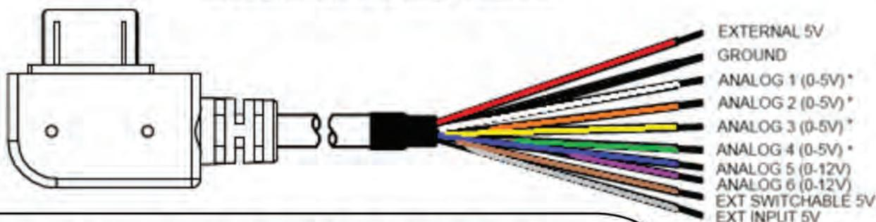
**Note: Minimum voltage for SCT analog 5, 6 & 7 is: 0.23V DC**
